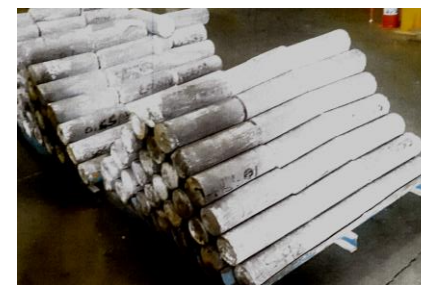
Cast billets ready for extrusion
