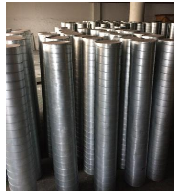
Canisters and spacers for MMO Titanium anodes used mainly on Pipelines
